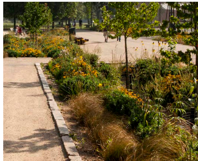
Figure 43 Sustainable Urban Drainage including rain gardens, within the design of public realm.
