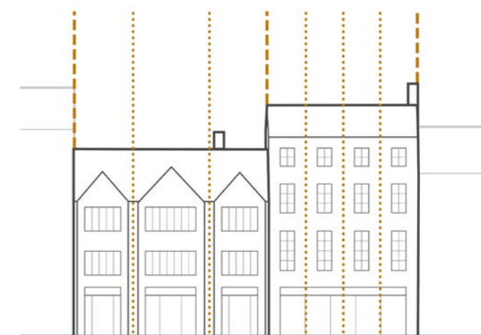
Figure 58 Verticality Within Buildings: Elevations divided into vertical segments to create a vertical rhythm.
